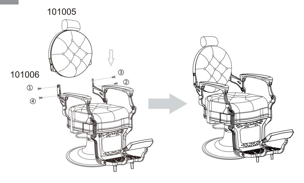
First tighten 1 to 4. Do not tighten them all at once. Wait until all 4 screws are aligned before tightening the 4 screws
