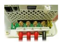
Up to 3 isolated outputs. Each output can carry the full current rating of the charger. However, not all simultaneously - the total current is the charger's rating.
