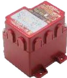
**Analogue VSR:** The Analogue VSR is the most affordable VSR that Sterling does. It has no adjustable features. The user can not adjust the voltage thresholds and there is no switching delay. The unit is also not 12V / 24V auto select. They are simply 12V or 24V models. The unit has a fixed on voltage of 13.3V and the fixed off voltage of 13.0V. Ignition override is also possible.
