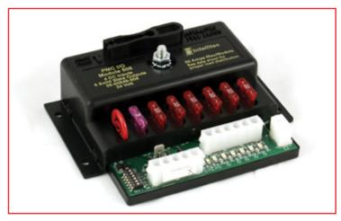
A Red LED Illuminates when power is applied. When multiplex communications are present and correct, the COMLED will Illuminate.
