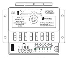
Turning switch 5 on causes Output Ch 5 to be operated directly from Input Ch 7 (acts like a Relay) Turning switch 6 on causes Output Ch 6 to be operated directly from Input Ch 8 (acts like a Relay)
