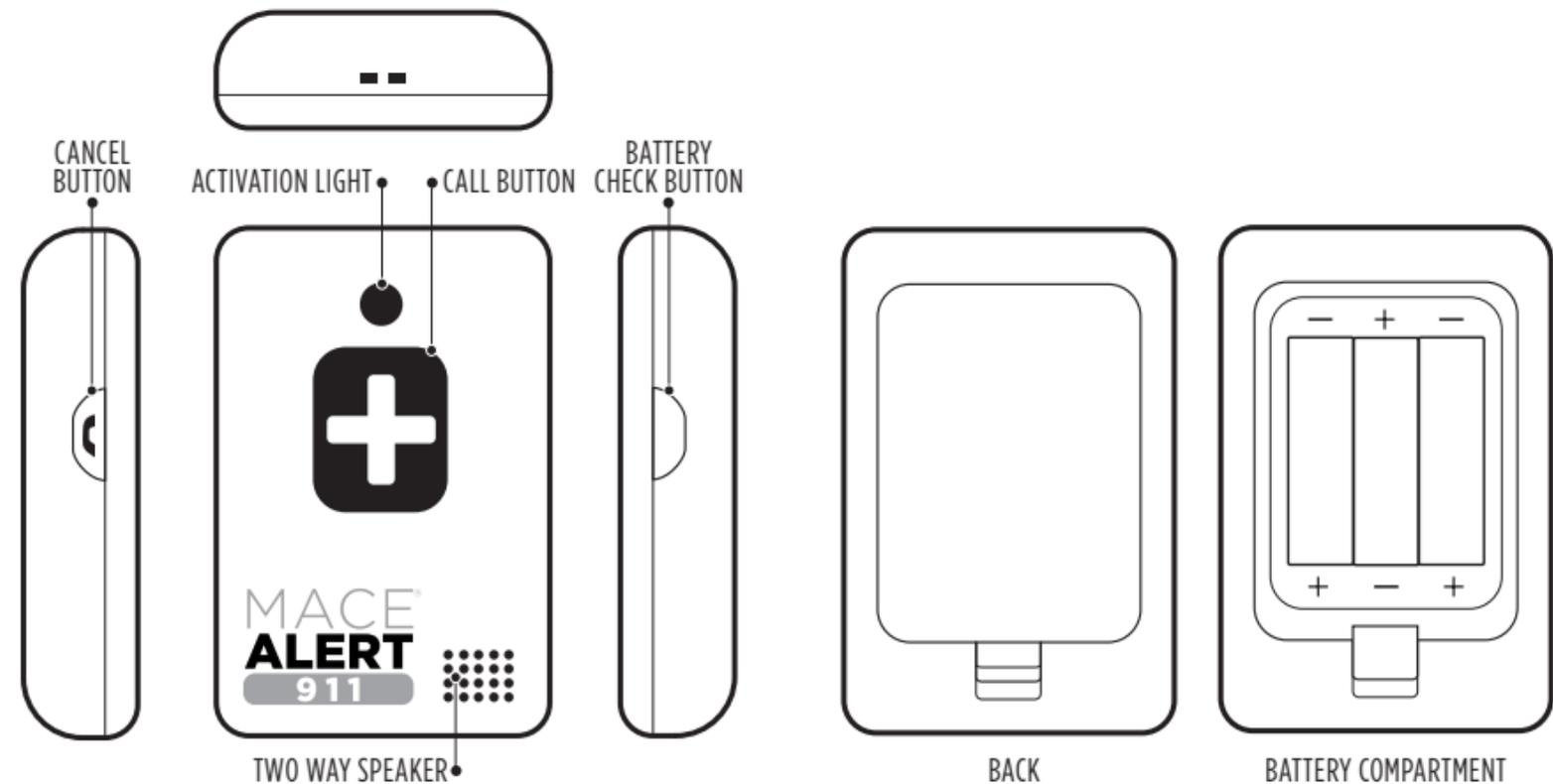
1. Open the battery compartment located on the rear of the device and insert three AAA lithium batteries (included). Take note of the polarity marking (+ / -) on case. Reattach the battery cover.
